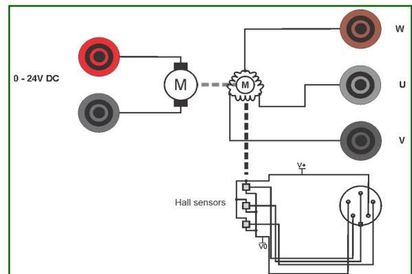
Unloaded, the brushless DC motor will generate 6V<sub>RMS</sub> between two phases at 2000 rpm.
