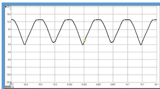
Notice that, after rectification, the peaks are spaced apart at half the signal period i.e. the full-wave signal has twice the frequency of the AC supply.
