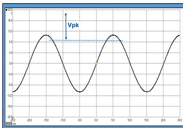
The RMS value, 6V, does not leap out as an obvious characteristic of this trace.
