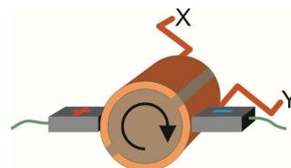
The pictures show a typical design of carbon brush, and a DC electric motor rotor with several windings. Its rotor contains a large number of coils, and so requires a more complicated commutator.
