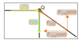
Force  $F_{CG}$  is again resolved into horizontal and vertical components.
