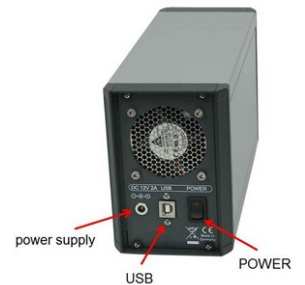
Fig. 13: Connectors at the back of the control unit
