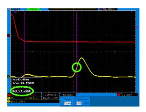
If you use the cursor function, the time of flight can be read off the screen as the difference between the two arrival times.
