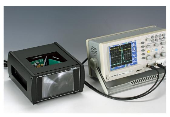
Setup with an older digital oscilloscope. The reflector is positioned outside the image.
