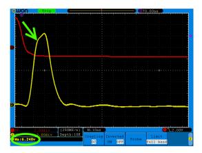
The image above shows a pulse that is distorted due to a too strong signal. (Max voltage measured: 6.24 V)
