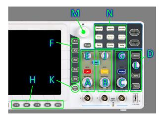
Buttons  $\mathbf{F}$  and  $\mathbf{H}$  are used for selections within menus that appear on the screen.  $\mathbf{M}$  is a dial, also used for selecting options shown on screen.
