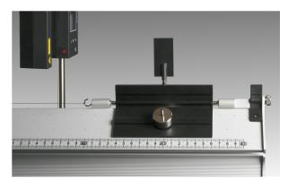
The length of the thread is chosen to let the weight pull the cart as far as possible. This means that when the cart is flush with the end stop, the loop is just clear of the pulley.
