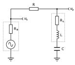
Use  $R = 500 \Omega$  (achieved by coupling two 1 k $\Omega$  in parallel) – se figure (c)
