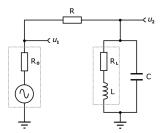
The parallel resonant circuit has an impedance maximum at its resonance frequency; a signal with a frequency further away will be damped.
