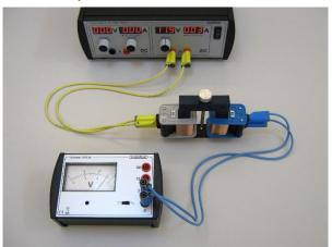
Power supply with a built-in voltmeter for measuring the primary voltage, and an external meter for the secondary voltage.
