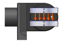
You can check this with a small magnet with known polarity. *Note: use a plastic-coated magnet (like 330850) in order to avoid damaging the neodymium magnets.*
