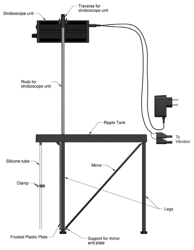
The propagated waves and patterns may be projected onto various surfaces. So far an oblique mirror has been used to project the patterns onto a frosted glass plate perpendicular to the ripple tank. This type of projection is well suited for demonstration and for group projects.
