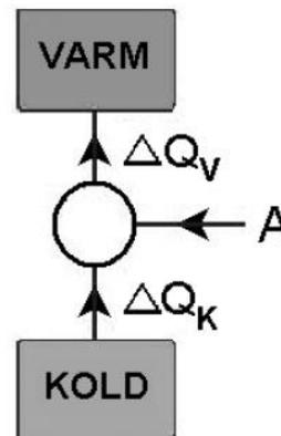
You can also consider the equation as a power equation, since  $A$  is understood as the power output (energy per second). In this ideal case, ignoring energy losses, etc.,  $\Delta Q_V$  will be transferred to an area where is a heat requirement while
