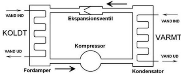
The compressor forces an appropriate fluid from the evaporator to the capacitor, a region of higher pressure and temperature (TV). The fluid is forced further through an expansion valve. The pressure and temperature decrease, and the evaporator is an area at lower temperature (TK). The two heat exchangers shown in the figure allow heat energy from the surroundings to be transferred to and from the heat pump.
