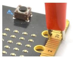
Connecting the alligator clips like this prevents any accidental connections between the large connectors with the holes in and the much smaller connectors (gold lines in the photo above)
