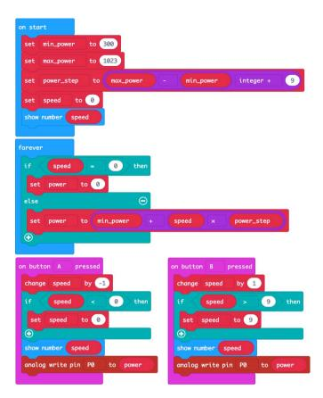
The *on button pressed* blocks are very similar to each other. The one for button A subtracts 1 from *speed* while making sure that *speed* does not fall below zero and then displays the new *speed* and uses *analog write* to set the power output of pin 0. The on button pressed for B does the same kind of thing, but adding 1 to speed.
