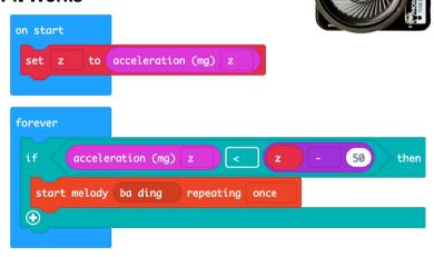
The program uses the micro:bit's built in accelerometer to measure any force acting in the z dimension (vertically). If the micro:bit is lying completely flat this will be -1023, but when the micro:bit is picked up, the force will change.
