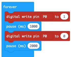
First Pin P0 is turned on using a digital write block. The 'pause' block then ensures that it stays on for 1000 milliseconds (1 second) before it is turned off. There then follows another pause of 2 seconds before the cycle repeats itself.
