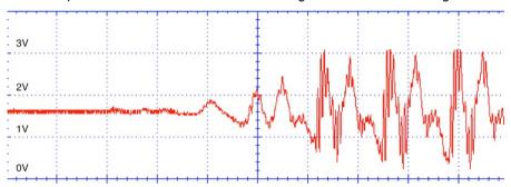
The voltage at the microphone output of the sensor board will always be between 0 and 3V, the signal swinging above and below a midpoint of about 1.5V. The number of LEDs lit is calculated from how much this signal voltage is above the signal midvoltage (1.5V).
