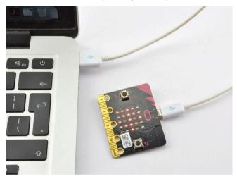
If your micro:bit is new, then its LED display will start displaying messages and showing off various features of the micro:bit. You are going to replace this program currently running on your micro:bit with a new one.
