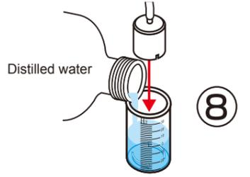
**Procedure for repeated gas production (after step 14):** Disconnect the small plugs from the tubes connected to the nozzles on the reversible fuel cell. This will allow water into the inner cylinders to replace the gasses and reset water levels to "0" line. Re-insert the plugs into the tubes and repeat electrolysis again.
