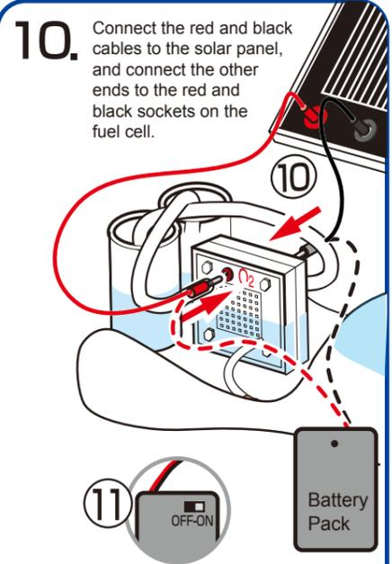
11. **ALTERNATE OPTION:** Connect the red cable from the battery pack to the red socket on the fuel cell and connect the black cable to black socket.
