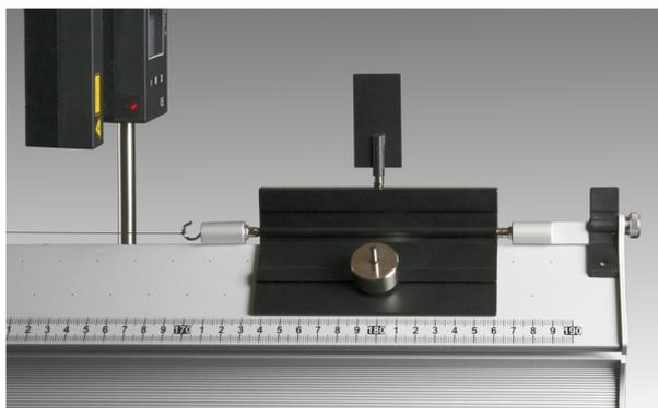
The length of the thread is chosen to let the weight pull the cart as far as possible. This means that when the cart is flush with the end stop, the loop is just clear of the pulley.
