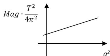
For comparison, the moment of inertia of the rod can be calculated by dividing it into a rectangular piece and two semi-circular ends – see the “Moments of inertia” section. The error of dropping a full treatment of the quadratic holes is quite small – but subtract their area when distributing the mass of the rod proportional to the areas of the three parts.
