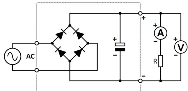
Now, the rectifier circuit is extended with a capacitor which is charged and stores the electric charge - which is given back again when the AC voltage is no longer big enough. Observe the polarity of the capacitor!
