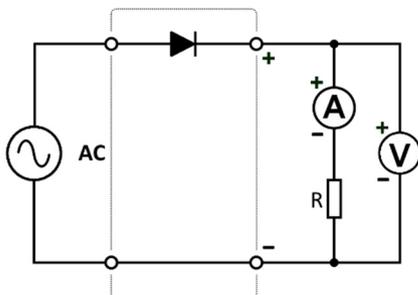
Insert a rectifier diode into one of the connections from the generator (the other is kept unchanged).
