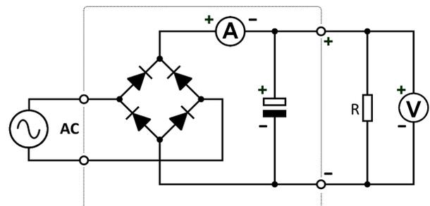
Instead of measuring the current through the resistor, this setup measures the capacitor's charging current. How does this current behave?
