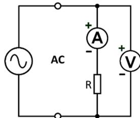
First, we will examine how the instruments behave when they are connected directly to the generator. Notice that the instruments are built to measure positive values – but they can also show a little bit below zero when the voltage or current is negative.
