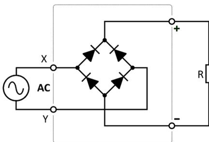
The AC voltage constantly changes sign, but we will study one instant where X is positive and Y negative. Take a colour pencil or marker and draw a line that follows the current through the rectifier and resistor *from X to Y* – take care to go only the right way through the diodes. You cannot go back to X – the current must go from X to Y. Draw arrows to show the direction of the current.
