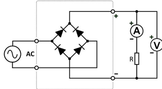
Exchange the diode with a bridge rectifier.
