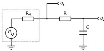
The cut-off frequency  $f_0$  of the filter is defined as the frequency where the signal is damped a factor of  $1/\sqrt{2}$  (i.e. about 71 % of the input voltage). It is given by
