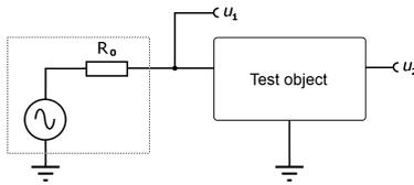
The signals at the input and the output of the filter are designated  $u_1$  resp.  $u_2$ .
