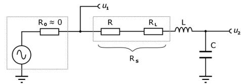
The setup resembles the previous; the only change is the use of the power output of the function generator where  $R_0$  can be ignored. The signal from the generator is fed to the input of the filter. Use square waves and a frequency of 5 kHz.
