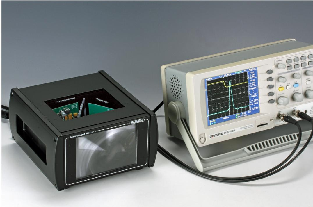
Setup with an older digital oscilloscope. The reflector is positioned outside the image.
