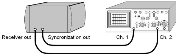
The following is a short description of the oscilloscope setup – for a detailed walk-through, see appendix.
