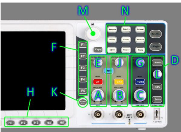
Buttons **F** and **H** are used for selections within menus that appear on the screen. **M** is a dial, also used for selecting options shown on screen.
