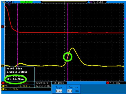
If you use the cursor function, the time of flight can be read off the screen as the difference between the two arrival times.
